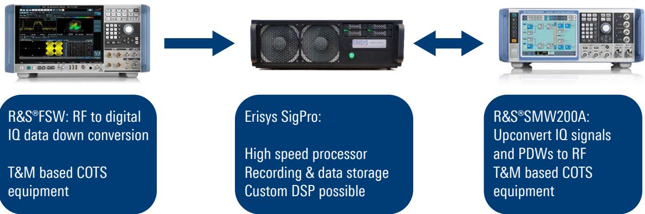
Figure 2: IRAPS functional description for each major component
