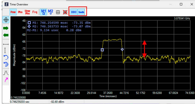
Figure 11: Same signal now with DDC processing applied - powerful processing shows as much as 30 dB improvement in showing the signal of interest
