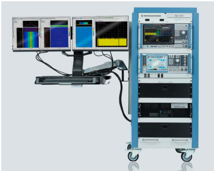
Figure 1: IRAPS configured in a rack system — includes 2 monitors with mouse and keyboard tray, and storage drawers for accessories. The main components for the IRAPS system are the R&S® FSW Spectrum Analyzer, the R&S® SMW Signal Generator, and the Erisys SigPro.
