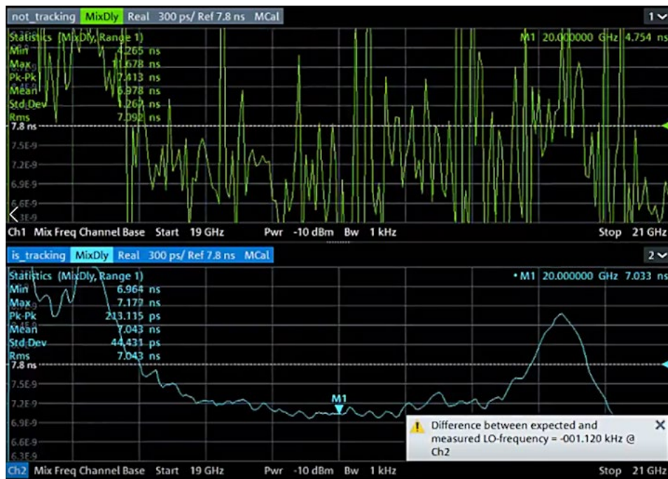
Figure 14. During a measurement of the satellite block downconverter, applying LO tracking (lower trace) provided a dramatic reduction in the noise and instability of the upper trace. The popup window (lower right) reported the measured difference between the actual and expected LO frequencies.
