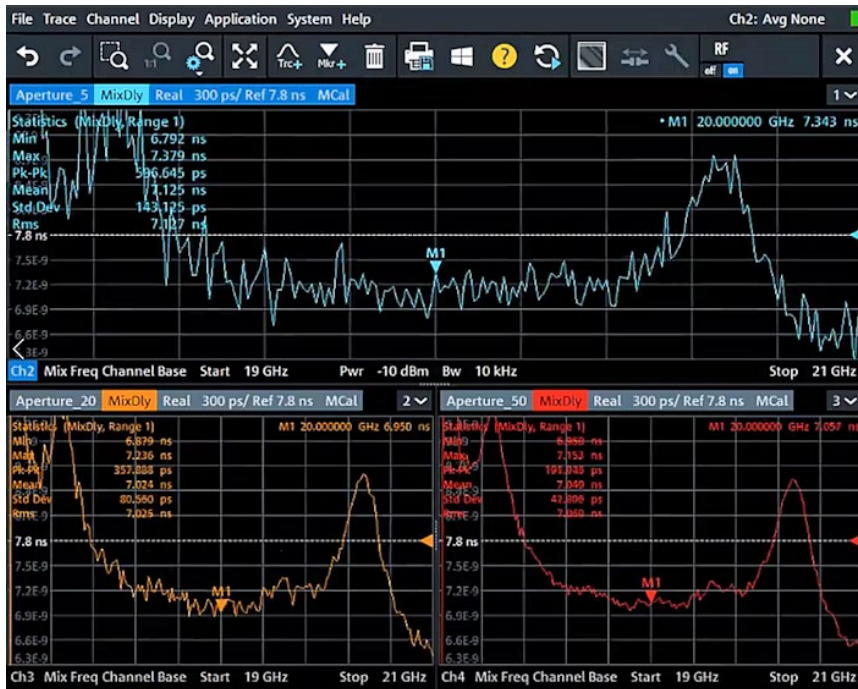
Figure 11. When measuring the satellite block converter, the consistent shape of the group delay measurement gradually deteriorated as aperture was decreased from 50 MHz (lower right) to 20 MHz (lower left) to 5 MHz (top).
