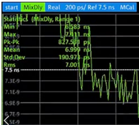
Figure 4. As shown in the table, the initial measurement of group delay through the satellite block converter had peak-to-peak variation of about 830 ps ("Pk-Pk" entry).
