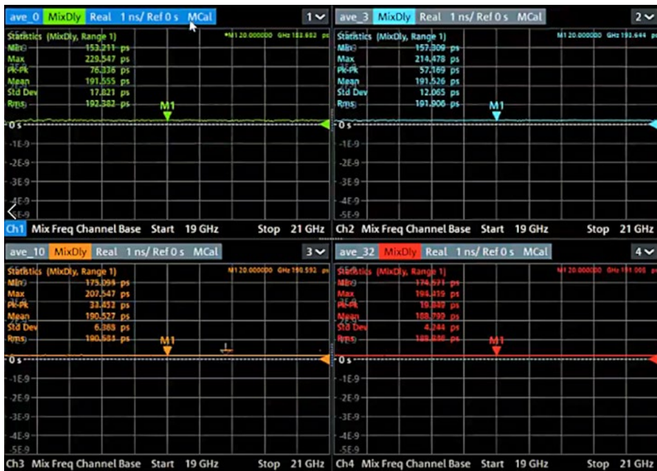
Figure 13. After considering the tradeoff between noise reduction and measurement time, using just three averages during calibration (upper-right trace) provides a meaningful improvement in peak-to-peak variation in group delay when measuring the calibration mixer.
