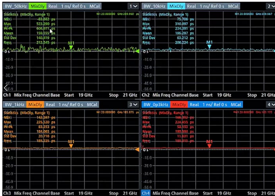
Figure 12. This series of measurements on the calibration mixer shows the reduction in noise at successively narrower IF bandwidths, proceeding clockwise from 50 kHz (upper left) to 10 kHz to 3 kHz to 1 kHz (lower left).
