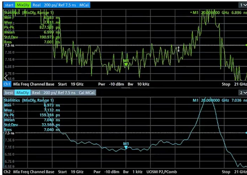
Figure 18. In the measurement of a satellite block converter, the tips presented here transformed a quick preset measurement (top trace) into a stable result with significantly improved peak-to-peak variation (blue table).
