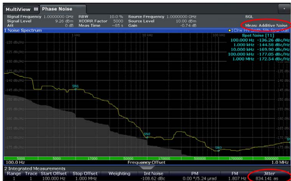
Fig. 2-3: Additive phase noise measured results.
