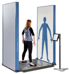
The R&S®QPS is a new high-resolution security scanner designed specifically to make people screening faster, more effective and comfortable at security operations. Utilizing safe millimeter wave radio technology, the R&S®QPS security scanner automatically identifies concealed objects and threats.
